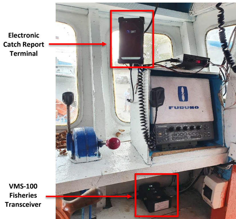
Philippine commercial fishing vessel equipped with VMS-100 fisheries monitoring system transceiver
