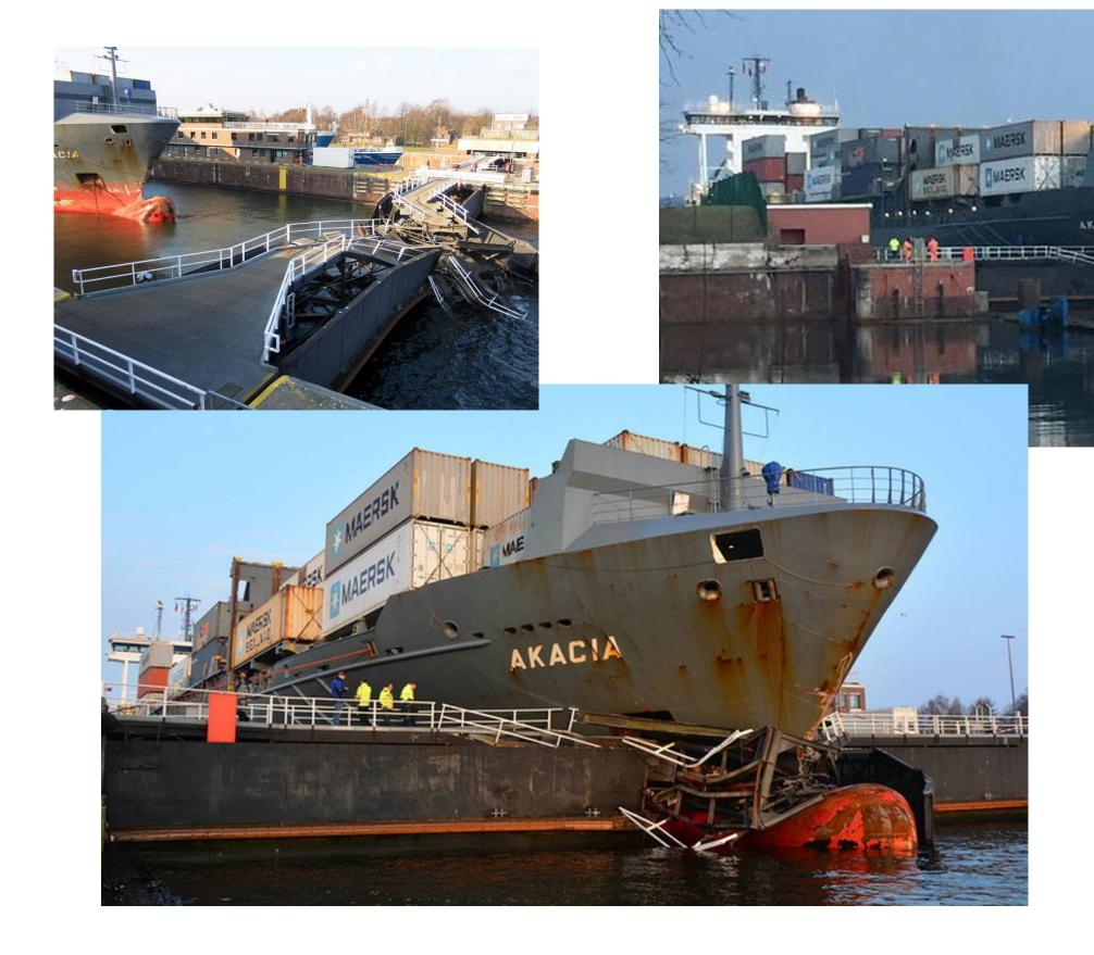
MV Akacia - hits closed lock. The ship and lock are severely damaged. DAS would help avoid this accident by transmitting the lock status in real time to the vessel, triggering alerts and allowing time to adjust speed to arrive at the right time.
